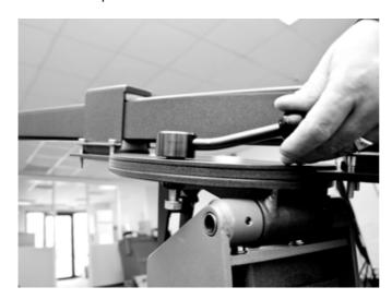
Pull the safety bolt down and check if the rotary moves are easy going. If it goes too strict, you have tightened the nut on the bottom too tightly.
