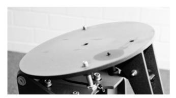
Unscrew the nut from the BOOM and put the BOOM on the bottom part as shown. The safety bolt, which is standing out from the bottom part, should be there where the holes are.
