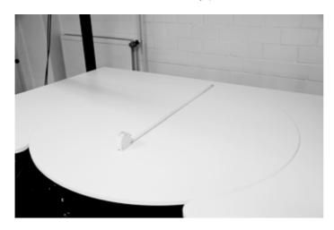
Screw the positioning pin with the attached brazing solder in the opening of the top-mounted rotary unit XY-TOP SPIN 300. The brazing solder should hang just above the mark of the rotary plate. So would be the XY-DESK in line with the rotary unit XY-SPIN 300, with the rotary unit XY-TOP SPIN 50. Pull the tread brake firmly to the DESK and the RACK.
