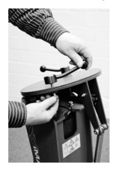
Tighten the screws so far that the ends overlap only appr. 5mm.
