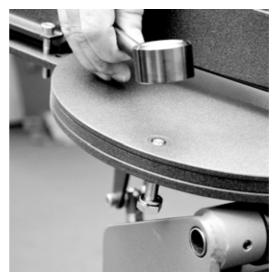
Place the lever screws and push them firmly down. Tighten the screws from underneath in the lever screw. Make sure that there is no space between the lever screw and the plate. If the screw is completely screwed in, the T-screw should be tightened. This is only possible when there is no space between the plate and the T-screw.
