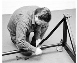
Connect the 3-point cross beam with the side parts as shown, insert the safety pins in the bolts.
