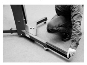
If the XY-BOOM is used with the XY-DESK, you have to mount the positioning help on the left lower crossbar of the XY-DESK. Screw the guide tight, only if you have positioned the robotic arm with the rotation axis to the center of the rotating plate of the XY-SPIN 300.
