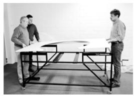
Place the plate on the DESK and look that it suitable fits. The edges of the frame may not stand in the circle cutout. As the desk frame is still not tight, you can make the alignment accordingly.
