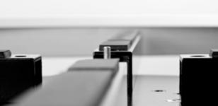
Put the plate carefully with the positioning hole on the rotary module. If the rotary module should not stand exactly in the middle, pull it to the right position until the plate slides easily on the positioning pin. Make sure that you can turn the plate easily. Screw the feet out as far as the plate has a slight protrude of appr. 2-4mm.
