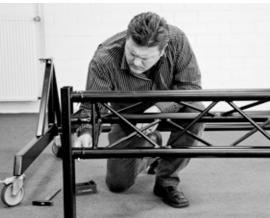
Measure out the exact middle of the 3-point cross beam. Attach the flange as shown lying still on the RACK-top, before you assemble the RACK completely.
