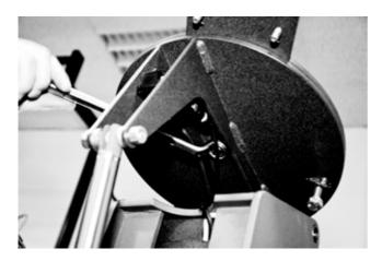
Put the cover panel with the holes right on the rotary module. Important! Make sure that the screws now have no more protrusion.
