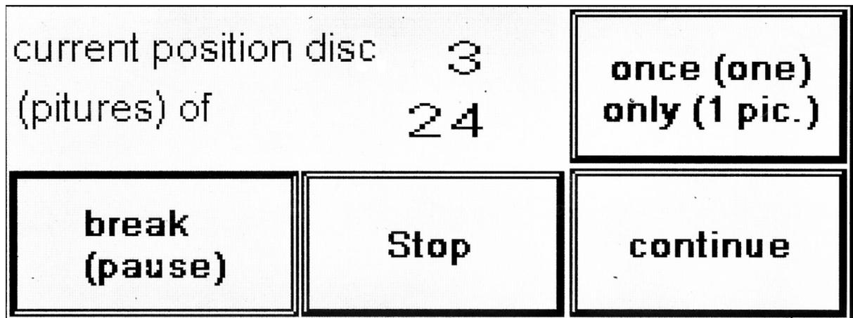
This shows the current image position and the total set quantity of the photos. Pressing the “**break**” button gives you the option of pausing the photography process. This is required if you would e.g. like to do an animation or make incremental changes in the photographed object. These can be realized quickly and easily with the “**once (one)**” button. Use the “**continue**” button to continue the process up to the specified photo quantity.
