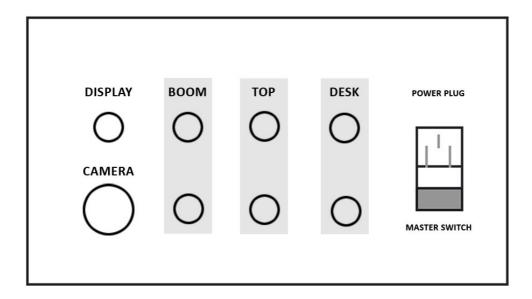
Make sure that the plug connections are always connected to the devices first, followed by the connections to the control unit. Connect the power plug to an electrical source listed on the identification plate.
