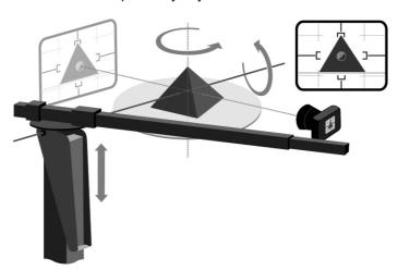
Adjust the axis exactly on the center of the object.
