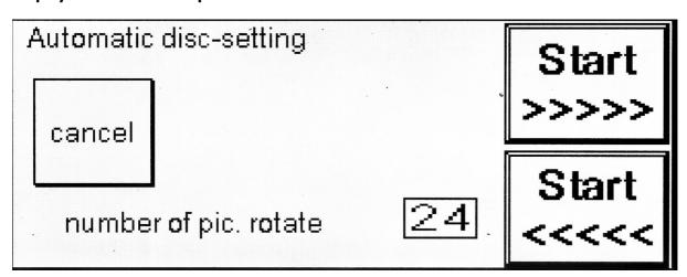
Press the button for the number of pictures to make a change or start the photography operation in the desired rotational direction.
