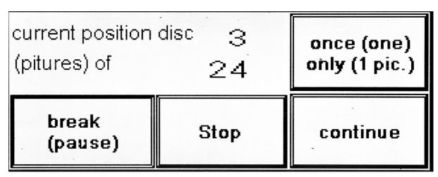
This shows the current image position and the total set quantity of the photos. Pressing the "break" button gives you the option of pausing the photography process. This is required if you would e.g. like to do an animation or make incremental changes in the photographed object. These can be realized quickly and easily with the "once (one)" button. Use the "continue" button to continue the process up to the specified photo quantity.
