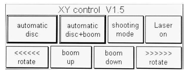
If you only use the rotating units without the robotic boom, the buttons "automatic disc, system, laser on, and rotate" are relevant for you. Only use the buttons "...boom" for the connected robotic boom XY-BOOM. If a device assigned to the buttons is not connected, an error message may be displayed. In that case, check the connections and restart the controls.
