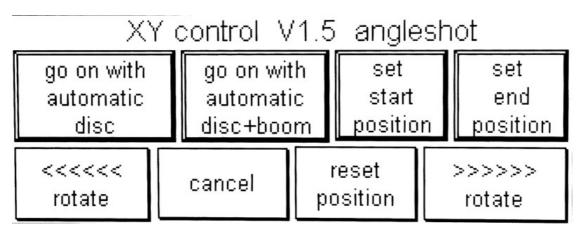
Turn your object into the start position, and set the start point, then turn the object to the end position, and set the end point. Press **"go on automatic disc"** the turntable automatically moves into the start position. Type the number of image and press **"start"**
