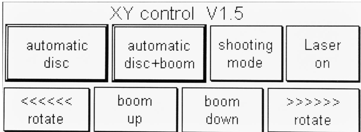
If you only use the rotating units without the robotic boom, the buttons “**automatic disc, system, laser on, and rotate**“ are relevant for you. Only use the buttons “...boom” for the connected robotic boom XY-BOOM. If a device assigned to the buttons is not connected, an error message may be displayed. In that case, check the connections and restart the controls.
